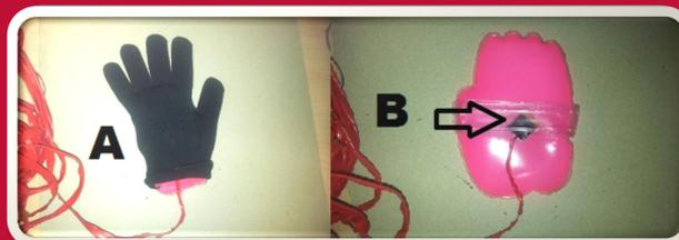
Method One: Typical arrangement of a heat pad inside a glove (A). The sensor was held in place using the heat pad "built in" strap (B).
