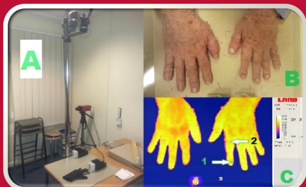
Method Two: The typical set up of the infrared camera for viewing hands (A). Images B and C show the hands of one of the subjects as viewed by the naked eye (B) and through IR imaging 5 minutes following provocation (C). NB this subject had neurofibromatosis.
