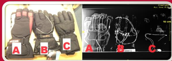
Heated Gloves (A= high range, B= mid range, C= low range) and X-ray Image of the Internal structures. Note the diffuse placement of elements.
